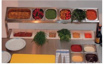
The table height can be adjusted electrically from 855 to 1155 mm. This always provides the ideal working height for both small and tall people.
